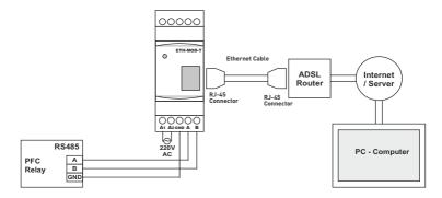
Only reactive relay or together with counter and energy analyzer can be connected with GSM-MOD on remote communication. Remote connection is made with reactive relay via www.tenseenerji.com (server) by connecting modem.
