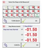
In order to reach step measurement (automatic measurement) page, enter these menus subsequently;
