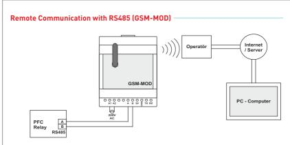
Only reactive relay or together with counter and energy analyzer can be connected with GSM-MOD on remote communication. Using a 100MB (recommended) data line from GSM operators, remote communication is made with reactive relay via www.tenseenerji.com (server).
